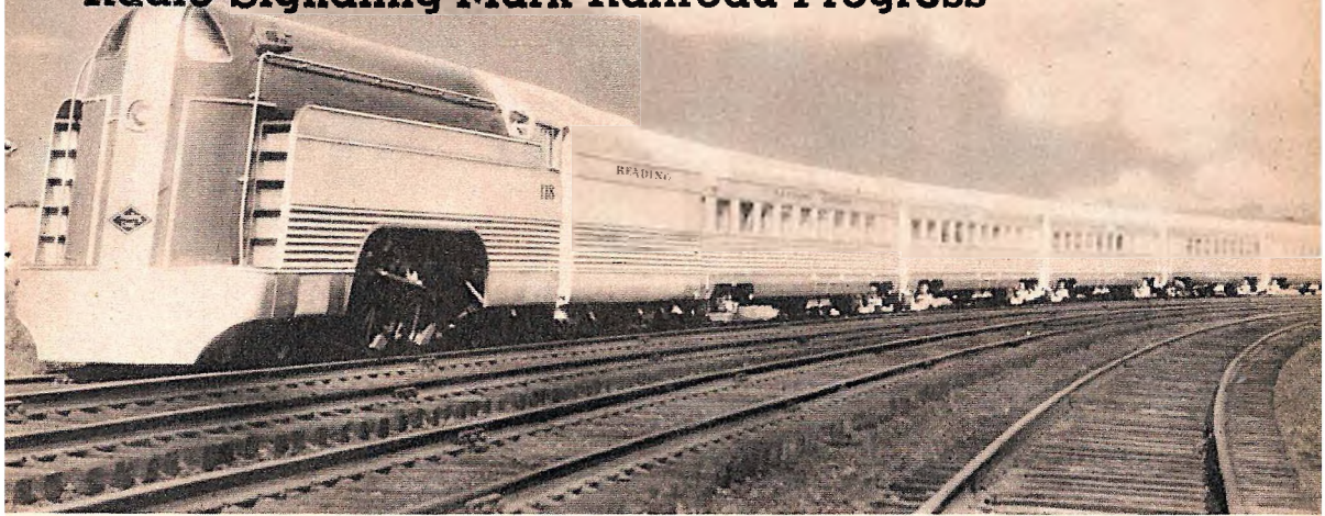
Flashing over the rails between New York, N. Y., and Philadelphia, Pa., this new streamlined train is the last word in passenger service and comfort. Except for wheels, axles, and truck assemblies, the entire train is constructed of stainless steel.
