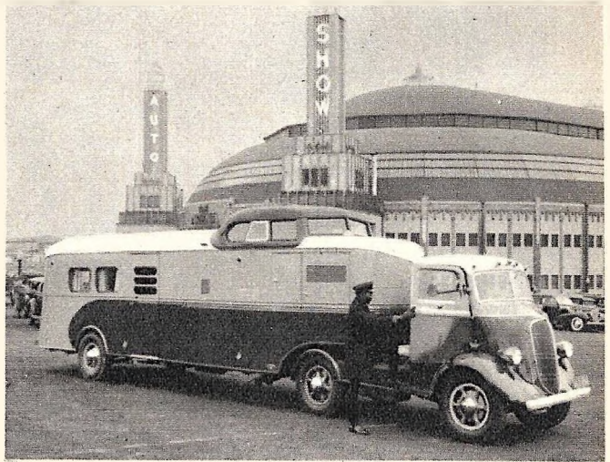
Note the special observation tower in which four persons can ride. It serves as sleeping quarters during the night for the crew. The trailer itself measures twenty-eight feet, while the trailer and tractor together are thirty-six feet long.
