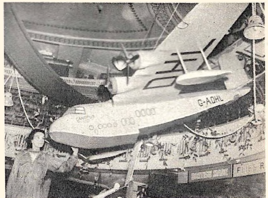
Equipped with four miniature gasoline engines, this replica of the Imperial Airways' flying boat Canopus is claimed to be the largest airplane model in the world. Wingspan is 15 feet.
