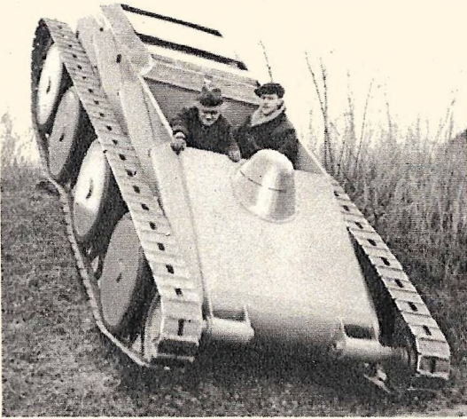
Weighing seven tons, this new type war tank not only climbs embankments with ease, but travels over level ground at a speed exceeding 50 m.p.h. Note how belt teeth engage wheels.
