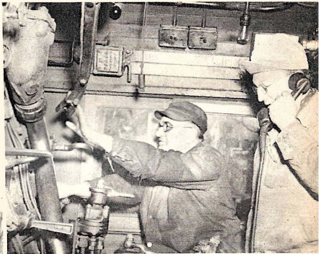
Freight trains go modern, too. Shown above is a scene in a locomotive cab as a crew member talks over a short-wave radio system to fellow workers in a caboose at the end of a long freight train. Left—Rigid aerial mounted atop caboose roof.
