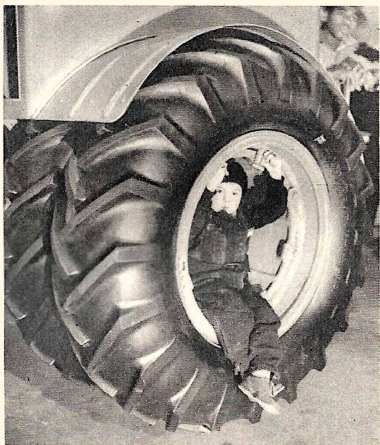
This giant tire is one of many which were designed and constructed to replace metal wheels on road building equipment. Note depth of tread, indicating ability to "bite" into ground.
