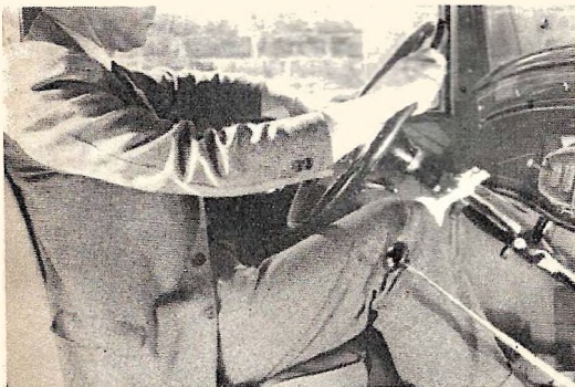
Easily installed on any auto, this knee-operated accelerator relieves strain of holding foot on usual gas pedal.
