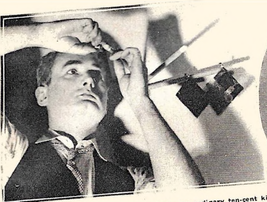
HANGER FOR DRYING CUT OR ROLL FILM. An ordinary ten-cent kitchen towel holder, which fits conveniently against the wall when not in use, will hold a dozen or so films while they are drying, as shown above. Attach each film to an arm of the holder with a push-pin, but do not crowd the films as they will dry more quickly if air can circulate freely around each one.
