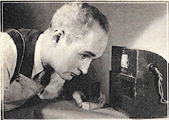
MIRROR REFLECTS LIGHT OF DARKROOM LAMP. With but one safelight in the darkroom, you can avoid carrying it about by using a small mirror mounted on a wood block, as shown above. This will reflect a spot of red light to any part of the darkroom. The angle at which to hold the mirror is determined entirely by experiment.
