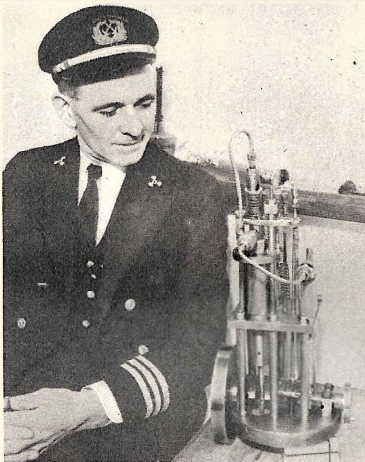
W. H. Greenfield, a marine engineer, proudly displays the tiny Diesel engine he constructed. Motor develops \frac{1}{2} -horsepower.
