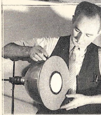
CONVERTING A FLOOD LAMP INTO A SPOTLIGHT. Cut a baffle from a piece of 1/4-inch Prestwood, placing bolts at the edges for hooking it over flange of flood lamp reflector. Cut a hole in center to accommodate a five-inch condensing lens and mount the latter, with convex side out, by means of Prestwood rings glued in place (left).
