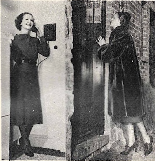
A compact kitchen telephone connected to a loudspeaker-microphone unit mounted on the outside doorjamb enables a housewife to identify callers before admission to the home.
