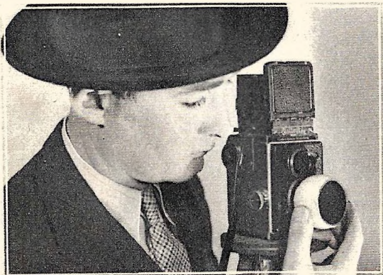
UNBREAKABLE LENS SHADE. Secure a five-cent rubber ball and cut an opening in one side for the lens and a larger opening on the other side. Blacken the inside completely with wallboard paint (below).
