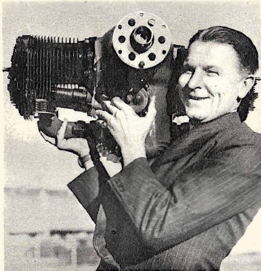
Capable of developing 50 horsepower at 2,550 R.P.M., this engine weighs 156 pounds and is only 27 \frac{5}{8} inches wide.
